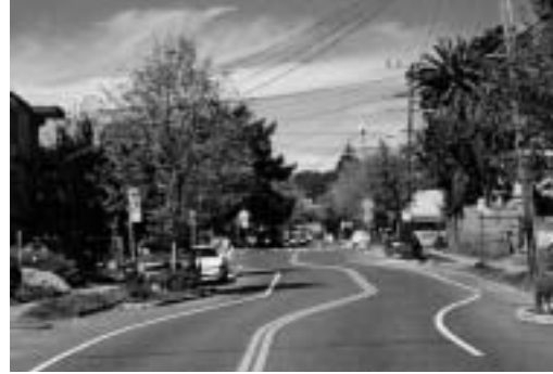
A chicane slows the speed of cars.
