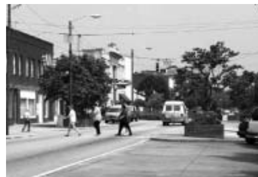
Curb extensions shorten pedestrian crossing distances and slow down cars.
